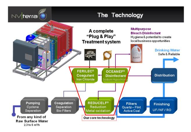
The mud resulting from the process is saved and can be used in agriculture in most cases, unless the treated water contained toxic contaminants (in which case the part of polluted mud is isolated). Trained staff on site is assisted in their maintenance tasks through the computer program that displays the progress of the operations and indicates the potential interventions. They are also assisted through the remote control system.
